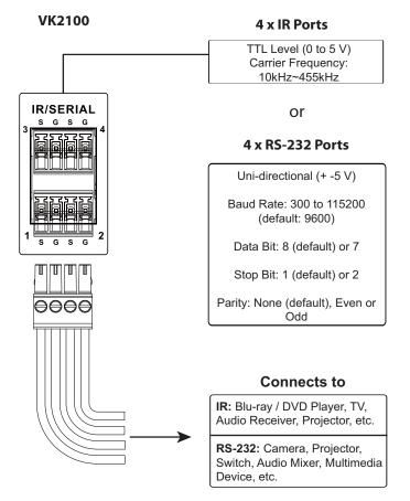
**IR Connection:** Connect a transmitter cable to the IR and Ground ports on the Control Box and install the IR transmitter on or near the device's IR receiving port, as shown on page 27.
