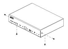
2. Use the two bottom screws removed in step 1 to secure the bottom of the brackets, and two M3X6 hexagon screws (included with the rack mount kit) to secure the side of the bracket to the VK1100.
