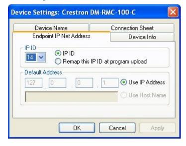
**NOTE:** The ID code specified in the SIMPL Windows program must match the IP ID of each unit. Refer to "Identity Code" on page 13.
