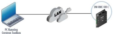
To establish TCP/IP communication between the PC and the DM-RMC-100-C via the **LAN** port of the DM-RMC-100-C:
