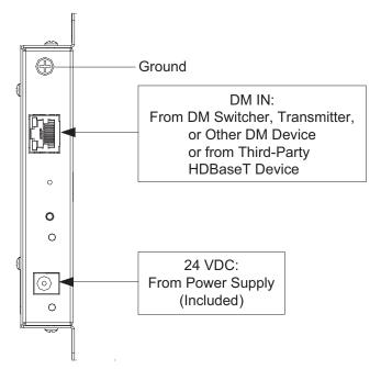
**NOTE:** Ensure that the unit is properly grounded by connecting the chassis ground lug to an earth ground (building steel).
