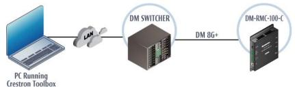
To establish TCP/IP communication between the PC and the DM-RMC-100-C via the DM switcher:
