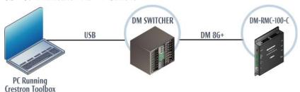
To establish USB communication between the PC and the DM switcher:
