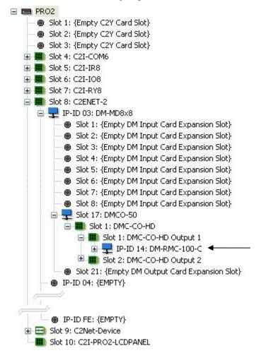
C2ENET-2 Device, Slot 8 (Using Ethernet Slot on Control System)
