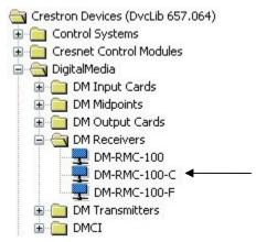
The system tree of the control system displays the DM-RMC-100-C in the appropriate slot with a default IP ID as shown in the following illustrations. In the first example, the DM-RMC-100-C is used with the DMCO-50 output card in a DM-MD8X8 switcher. In the second example, the DM-RMC-100-C is used with the C2ENET-2 card in an Ethernet slot on the control system.
