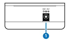
**DC 5V:** Connect to the 5V DC power supply into the unit and plug the adaptor to an AC wall outlet.
