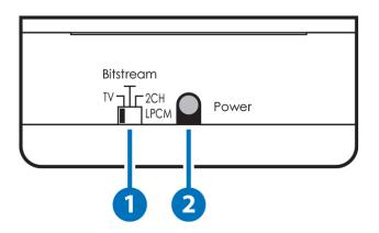
**TV/Bitstream/2CH LPCM:** This switch allows users to select the source's audio EDID.
