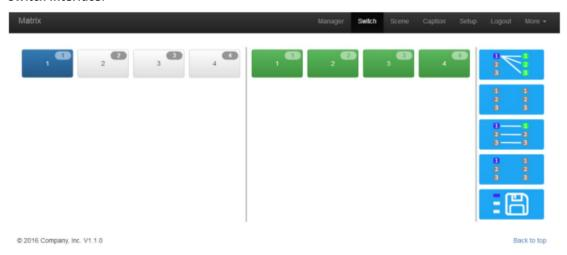
The left side of the long string is input area, the right side is output area, the buttons are the same with input area. And there're 5 buttons: The  $1^{st}$  for 1 to all,  $2^{nd}$  for 1 off to all,  $3^{rd}$  for 1 to 1,  $4^{th}$  for all off, the last one is for scene save and recall. (Change names can be done in Caption interface)
