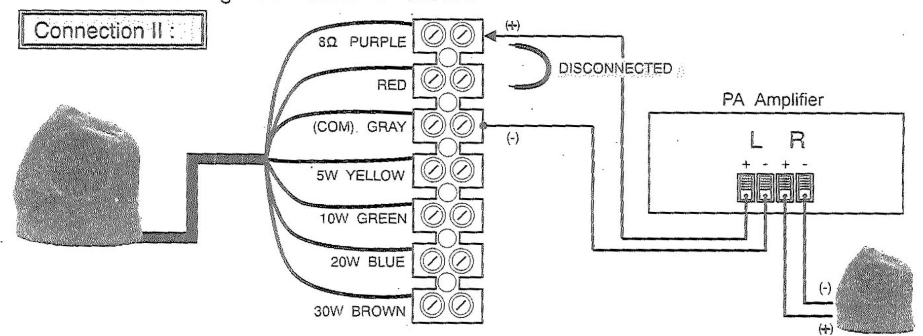
When connecting the loudspeakers make sure that the connecting cable is not squeezed or damaged by sharp edges.
