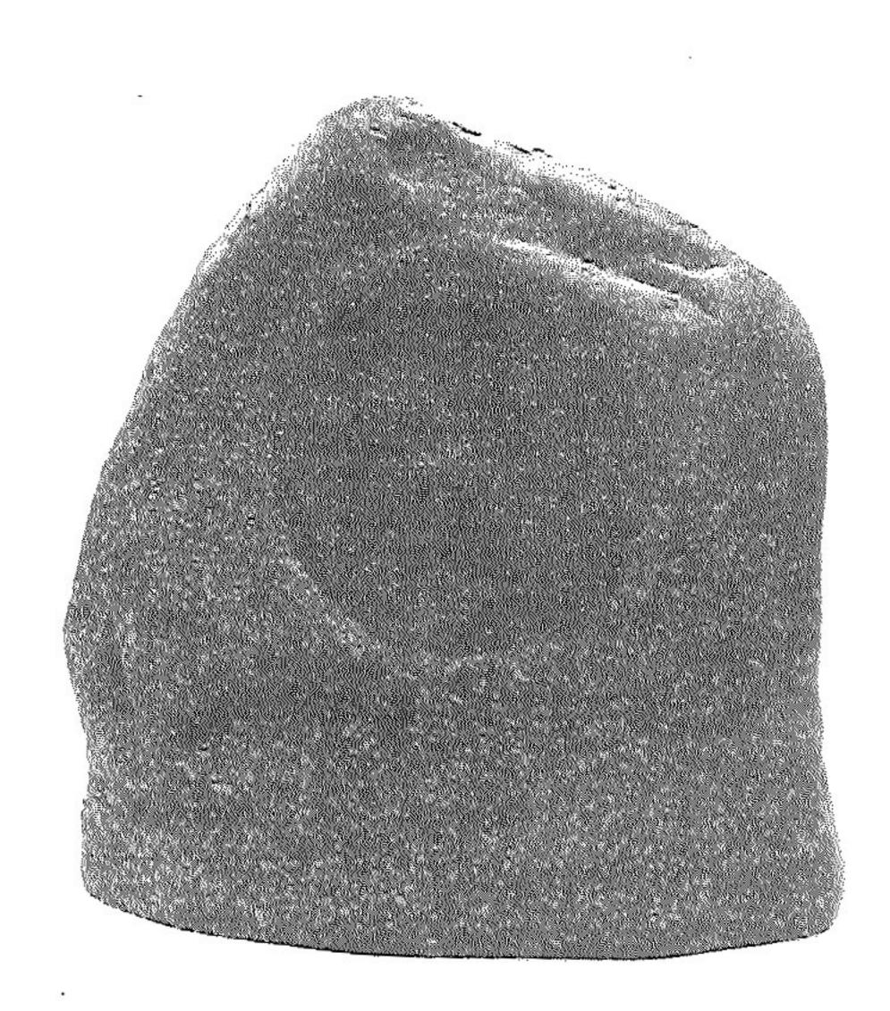
6.5 inch Garden Speaker Water Proof Two Way 6.5 inch Coaxial Speaker Built-in Woofer: 8 OHM, injection PP cone, Rubber surround, 25MM voice coil, Steel painting basket Tweeter: PEI dome/25mm voice coil/neodymium magnet system Transformer: 100V 30W/20W/10W/ 5W/8OHM, with the cable select the output
