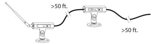
Use a maximum of two in-line antenna amplifiers for extremely long cable runs or for two runs of lighter-grade cable, as shown
