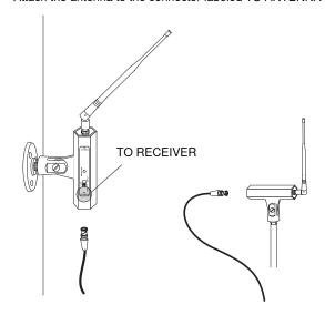
Use the supplied surface-mount bracket on walls or ceilings, or mount on a standard microphone stand.
