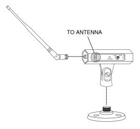
Attach the antenna to the connector labeled TO ANTENNA
