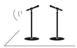
**Important:** Always perform a "walk around" test to verify coverage before using a wireless system during a speech or performance. Experiment with antenna placement to find the optimum location. If necessary, mark "trouble spots" and ask presenters or performers to avoid those areas.
